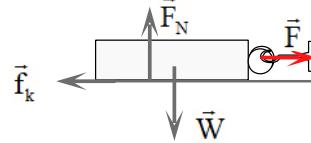
$$\begin{aligned} F - f_k &= ma \rightarrow F - f_k = 0 \rightarrow F = f_k \\ F = f_k &= \mu_k mg \rightarrow \mu_k = \frac{F}{mg} \end{aligned}$$
